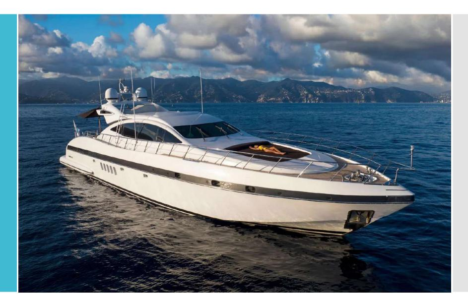
Built with a GRP hull and GRP superstructure, she has impressive speed and great efficiency thanks to her planing hull. Powered by twin MTU engines, she comfortably cruises at 25 knots, reaches a maximum speed of 36 knots. Her low draft of 1.2m/3'11" makes her primed for accessing shallow areas and cruising close to the shorelines.
